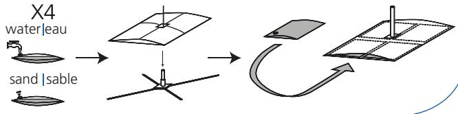
After the poles are attached to one another, insert them into the flag's sleeve. Then, wrap the elastic bungee around the plastic hook on the bottom pole. Finally, place it all onto the spindle and the base.
