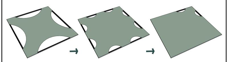
starting in one corner of the frame, tuck silicone edge of fabric into channel. Repeat for the other three corners.
