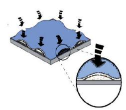
Work your way accross top of graphic tucking silicone edge into channel. repeat for the sides and bottom.
